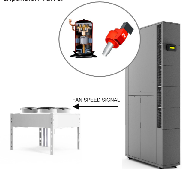
Example of connection between Ed+ unit and air cooled remote condenser.
